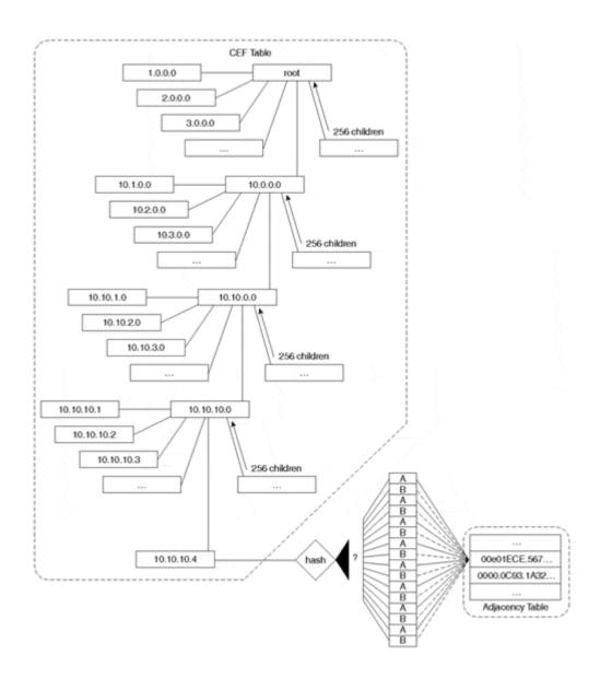
When the CEF switching method finds a load-share entry—rather than an adjacency table entry—as the result of a CEF table search, it uses the source and destination address to decide which of the entries to use from the load-share table. Each entry in the load-share table then points to an adjacency table entry that contains the MAC header and other information needed to forward the packet.
